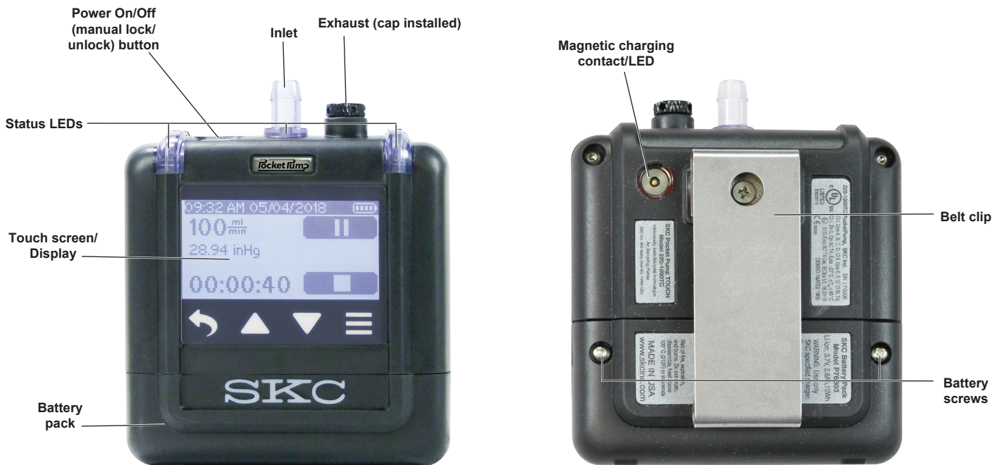
Figure 1. Pocket Pump TOUCH Physical Feature Overview
