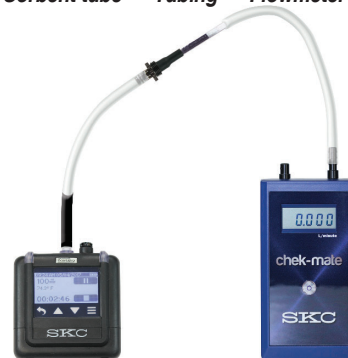
Figure 3. Single-tube Flow Verification Train Overview
